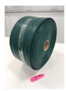
Drainbelt is 200mm wide and is supplied in 50m rolls weighing less than 20 kgs, making the product easy to unload and handle on site. It is simply rolled out on the graded sub-base. Drainbelt can be cut with a Stanley-knife/box cutter.
